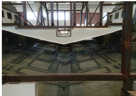
SCIGRIP's Methacrylate adhesives have been used for years in structural bonding applications in the marine sector, reducing surface preparation requirements and providing a versatile bonding system that can be tailored for the individual gap size and working time requirements of each job.
