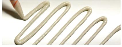
**SCIGRIP® SG350L Series** is designed for mixed material bonding applications with stringent aging resistance requirements. The ratio between open time and fixture time is advantageous as compared to other methyl methacrylate systems.
